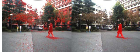
Fig. 3 Example of change detected (red). Left without discard of periodic changes. right discarding them.
