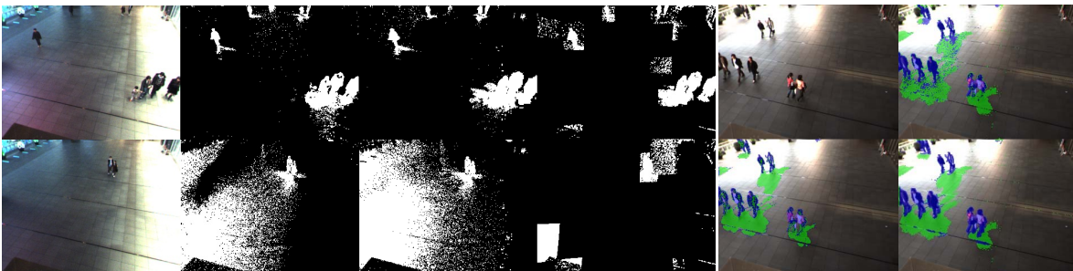
Fig. 5. Two frames of environment with light changes and presence of noise, Statistical method, codebook and proposed are compared.
